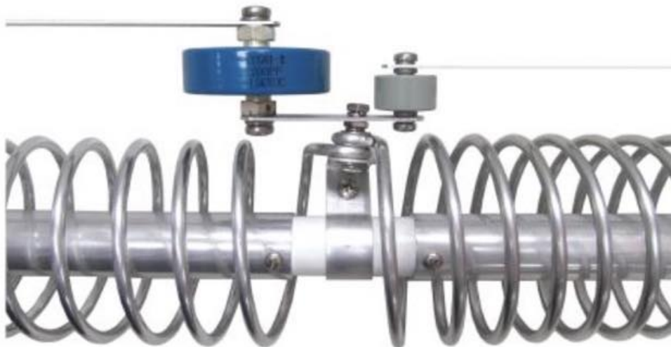
Figure 2. Closeup of a Butternut trap. This is very robust and low-loss design.
