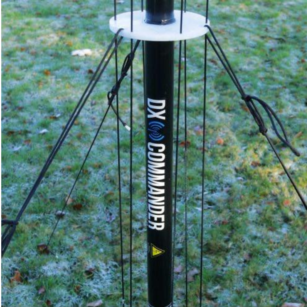
Figure 1. Detail of the wire guide/guy ring on a DX Commander vertical.
