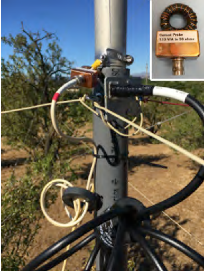
Figure 8. At the antenna feedpoint, you can see the mighty K9YC-approved choke on the phasing line. Inset: A temporary current transformer is connected via a (choked) test cable.
