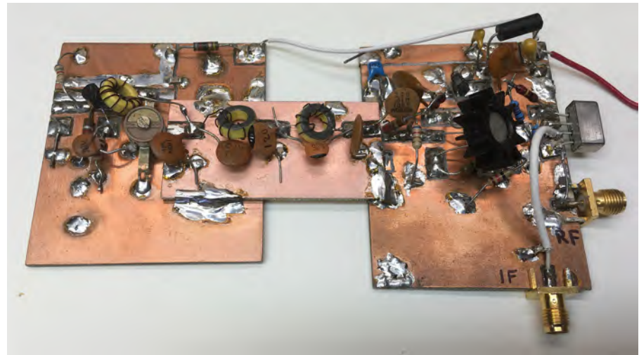
Receiver RF-IF chain built up from smaller modules. Build and test each one, then link together.
