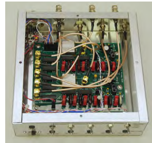
Lowband RX antenna filter and distribution
