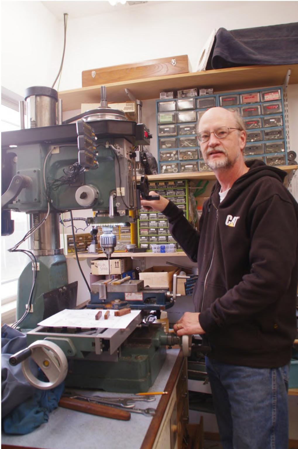
My Chinese drill-mill. This sow's ear has been turned into a silk purse by adding an adjustable-speed drive, digital readouts, spindle illumination, and a whole lot of careful adjustment.
