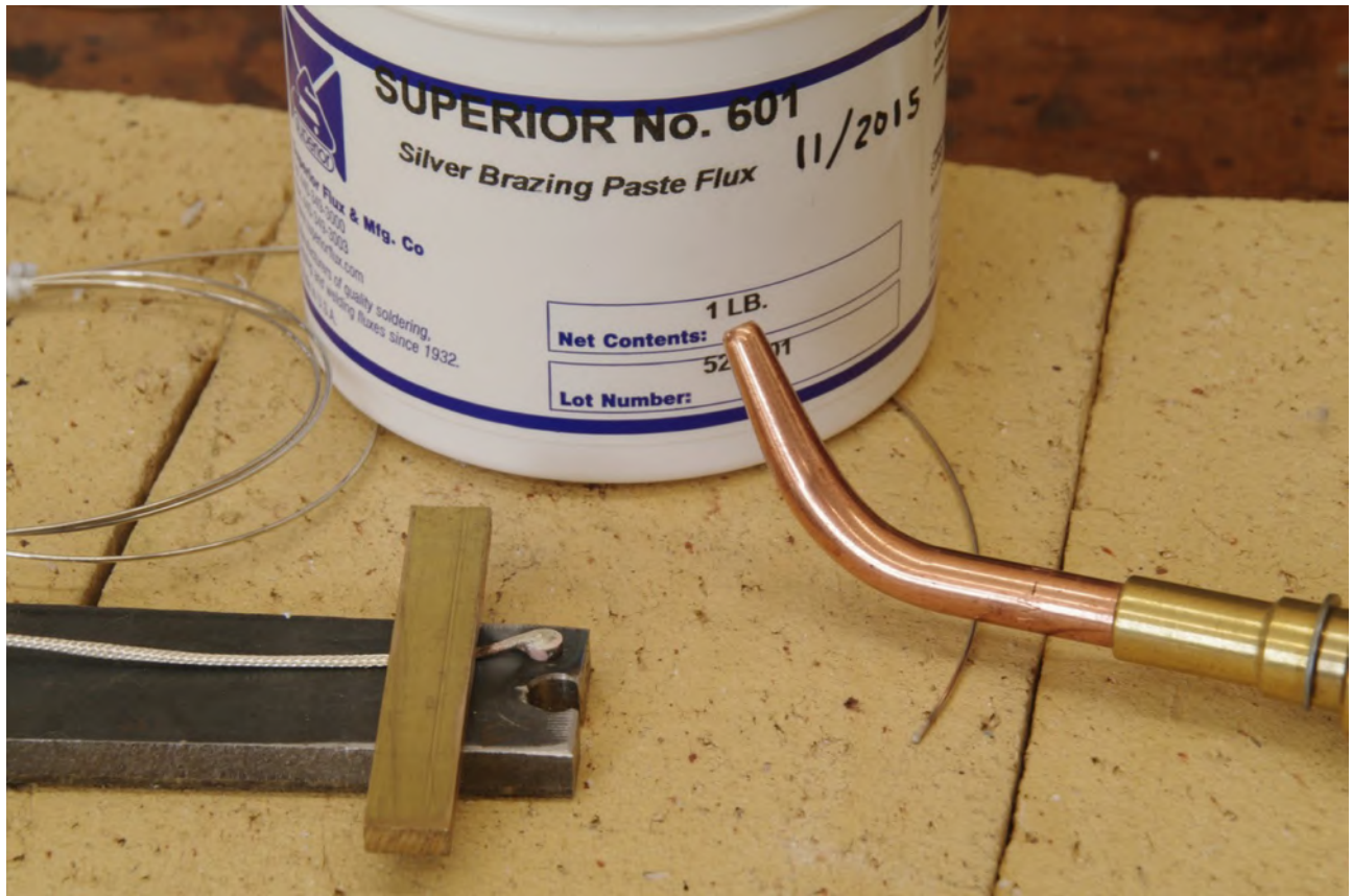
Silver soldering small braid to a dash contact. The parts sit in a fixture and the oxy-acetylene torch makes quick work of it. For the Model 2 Woodbug, I used the smallest size of solder wick for the braid.
