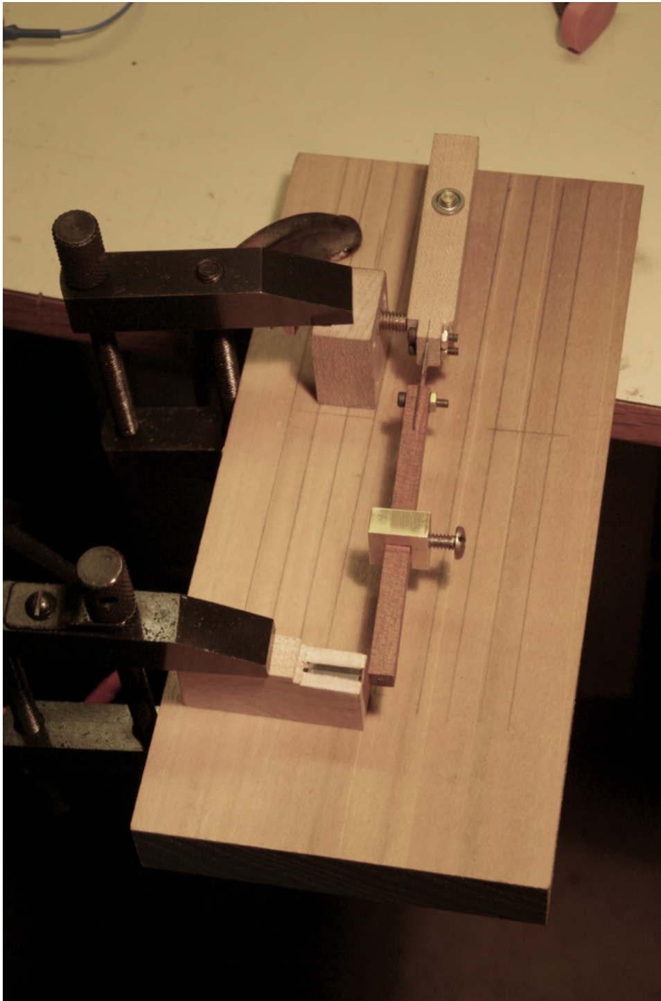
Component testbed. This was used to try out various mainsprings, weights, and in this photo, magnetic reed switches as the dot detector. I had also experimented with magnetic return springs but never liked the way they behaved.
