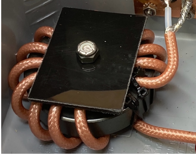
Figure 3. A toroidal choke clamped in place with a piece of 1/8 in. acetal and a machine bolt.
