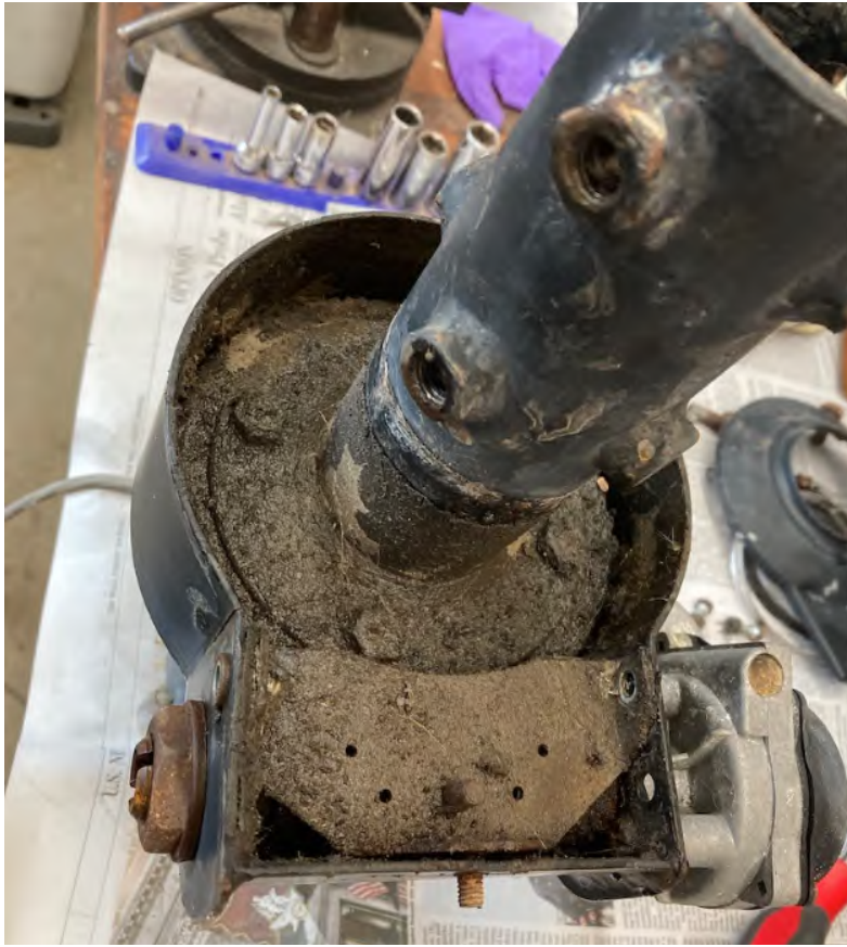
Figure 11. This Alfa-Spid RAK rotator definitely needed servicing.
