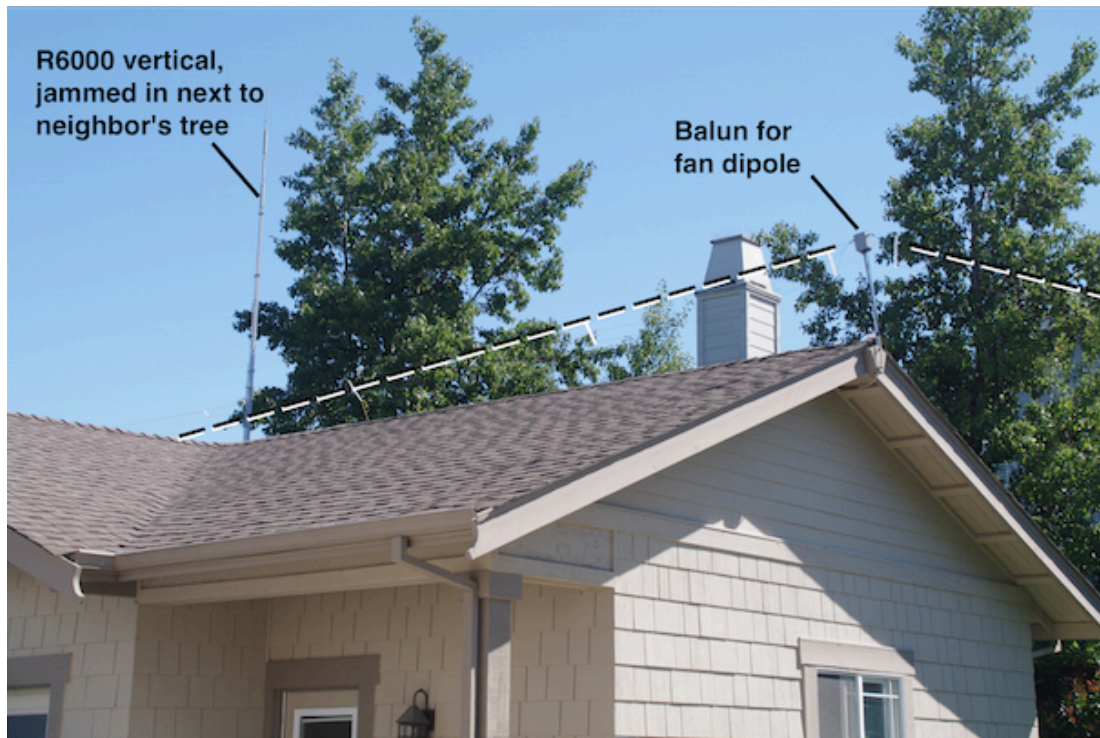
Figure 2. My primary antennas, a vertical and fan dipole. This is a flagrant violation of my CC&Rs, but I have yet to get caught.
