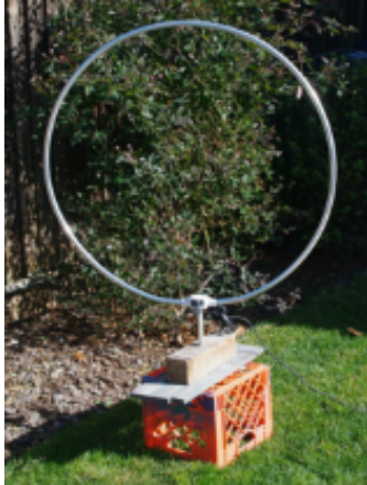
Figure 3. A magnetic loop antenna for receiving, oriented to null out the evil plasma TV next door. Note the sophisticated rotation mount and support structure.
