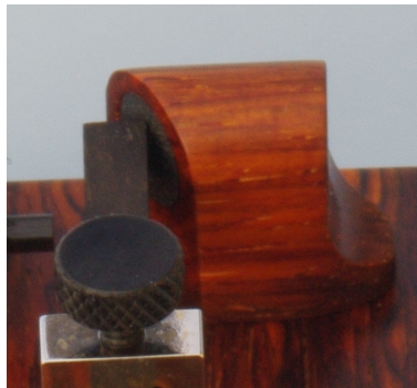
Figure 6. Closeup of the damper, with its soft polymer material mounted at an angle so as to maximize point force.
