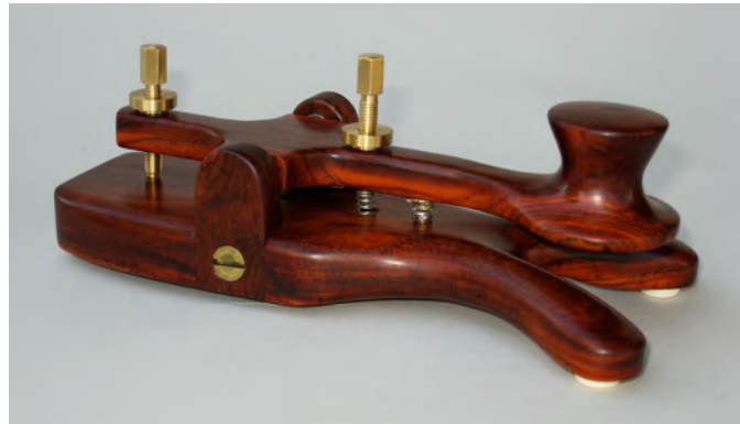
Figure 1. Morse hand key, made by the author in 2008. Cocobolo.
