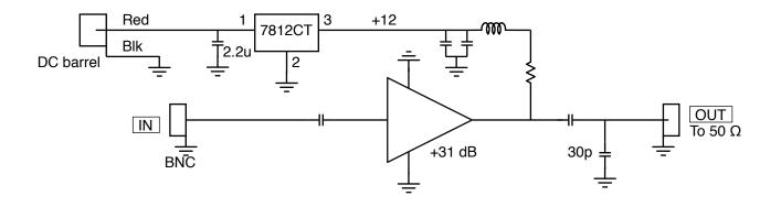
For HP 5384A frequency counter 10 MHz reference output (-20 dBm, square wave)
