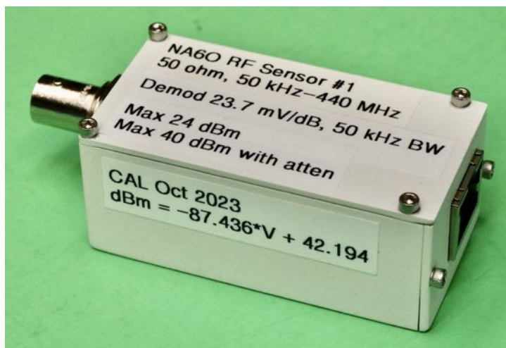
Figure 5. The completed RF sensor #1.
