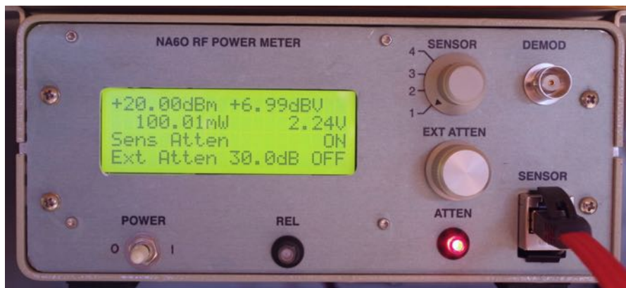
Figure 1. Front panel of the power meter controller.
