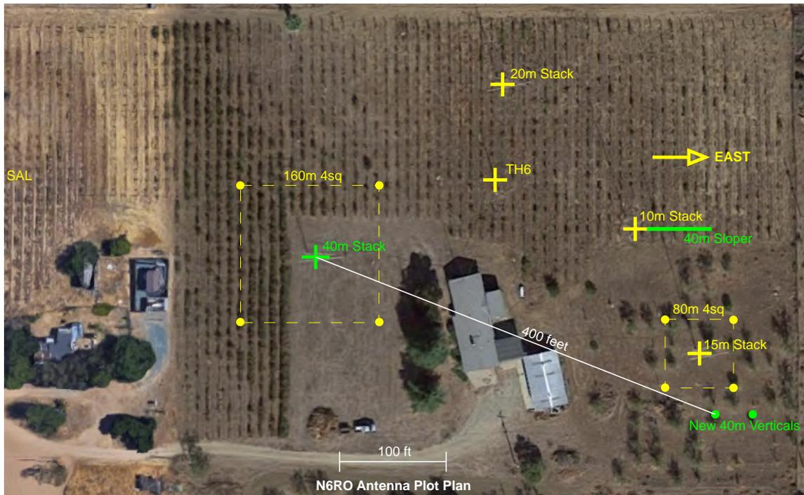
**Figure 1.** Plot plan, highlighting the 40 m antennas.
