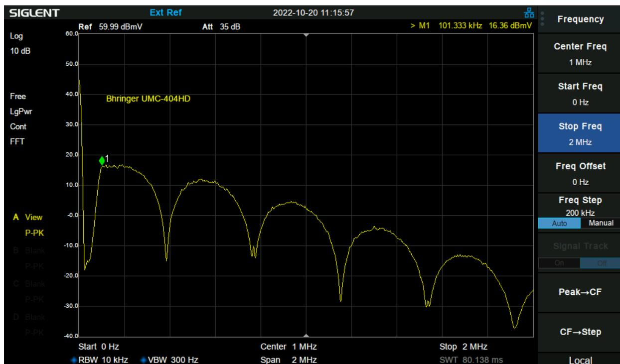
**Figure 4. Significant RF energy is present on all DAC outputs of this Behringer UMC-404HD.**
