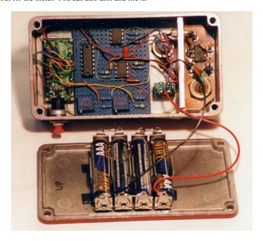
The RF section is walled-off at the upper right. I machined a piece of 0.125-inch aluminum to fit exactly between the inside walls of the case and then fixed it in place with #2-56 screws. The RF section circuit board is held in place by the BNC connector's nut. There are feedthru capacitors through the divider wall. The AD8307 is mounted dead-bug and lead lengths are absolutely as short as possible. That's why it works way out into the UHF region.
