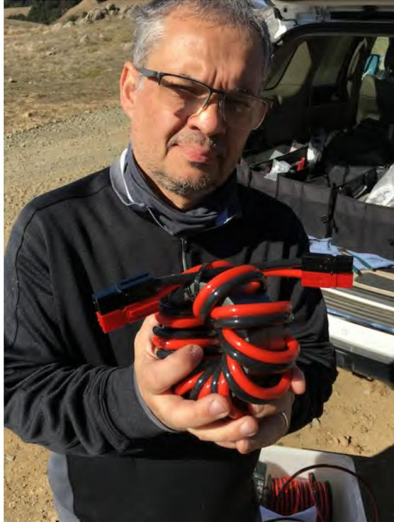
**W6TCP holding the high-current battery choke.**
