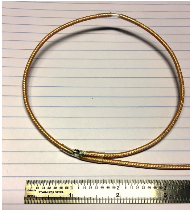
Figure 7. Completed pickup loop, about 3 inches diameter.
