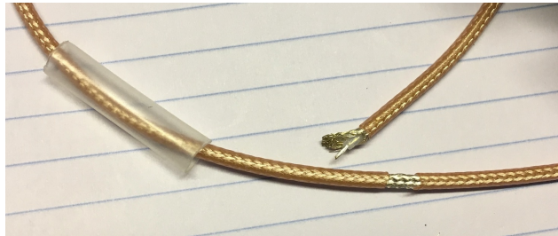
Figure 6. Ready to solder the loop closed. Heatshrink is in position.
