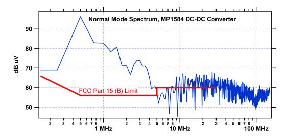
Looking at the input ripple, it contains fast spikes at the 243 kHz switching frequency and also some lower-frequency modulation. Spikes are 5 ns FWHM and ring down at about 150 MHz; additional spectrum analysis showed energy there.
