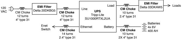
One-line diagram of RFI mitigation on the second UPS installation.
