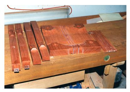
Here are most of the parts. Shaping the legs took a great deal of thought because of all the odd angles. Contouring is done after all the joints are cut, otherwise you have no means of registering the mortises and tenons.
