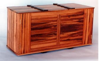
You can see the continuous grain on the drawers; the top and bottom also have pleasing grain lines since all parts were resawn from one large plank and then bookmatched. End doors are coopered to form a gentle curve. The back is frame-and-panel.
