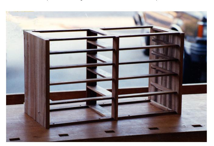
The carcase is also made from Goncalo Alves, with most of the pieces resawn to about 5/16 of an inch thick. Joints are mortise and tenon as well as some tiny dovetails. This is traditional carcase construction only scaled down. There are about 35 parts in it.
