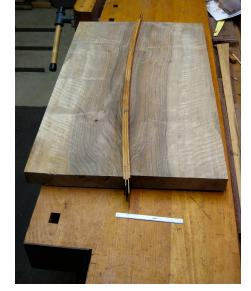
made from a twoinch slab, which had a nasty, curved crack right down the middle since it was cut right thru the pith of the tree. So I cut out that bad part, and laminated in strips of contrasting wood. Joining on the curve is challenging...
