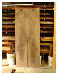
Nominal one-inch slabs were crosscut and then ripped into strips that would be glued up into the main side panels of the desk. The panels are coopered, requiring numerous strips. Also, flattening narrower strips reduces waste.
