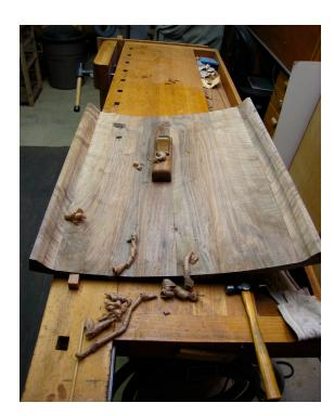
One end of the desk is supported by this curved, tapered leg. It's shaped with a curved plane (among other tools). Below, I'm getting ready to cut a series of tenons where it mates with the top.
