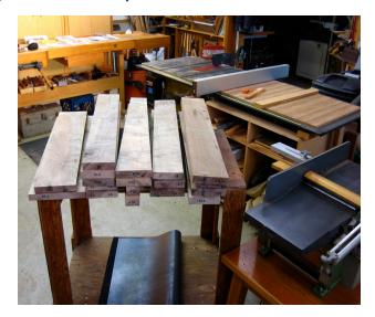
Here are the parts for one of the sides. Beveled at 2 degrees, the form a 5-foot radius when glued up. A total of five such panels (two of them coopered) occupied all my clamps for quite a while.
