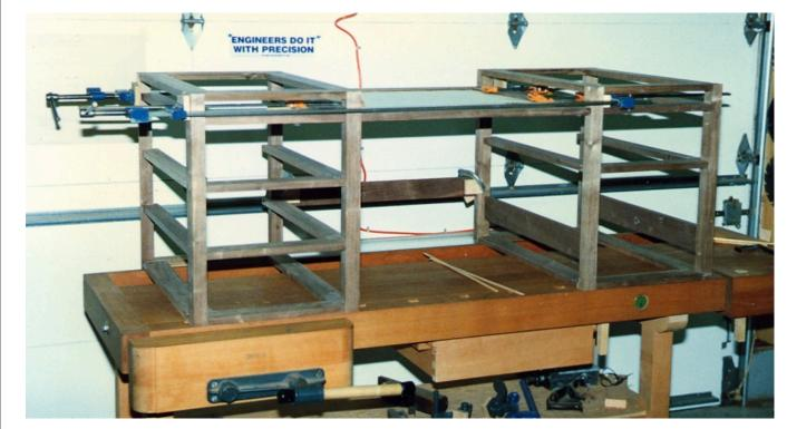
Here is the carcase, during glue-up, showing traditional frame-and-panel construction. Joints are mostly mortise and tenon with a few dovetails.
