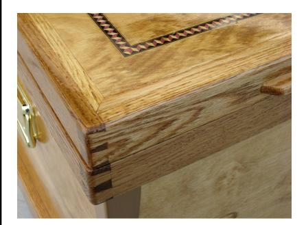
There is commercial inlay on the top. Finish is a Watco Light Walnut and four coats of alkyd spar varnish on the outside, and waterbase polyurethane on the inside.
