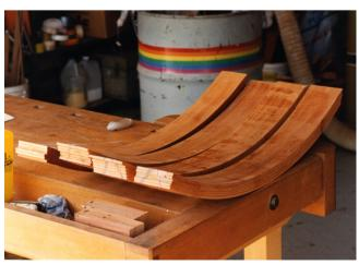
Legs are bent laminations. Many layers of Mahogany were resawn on the bandsaw to about 3/32" thick. A curved set of forms was built from two-by construction lumber.
